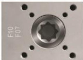
Bottom mounting connection is designed in accordance with ISO5211 and DIN3337 standards for direct mounting with valve gear boxes or mounting brackets
