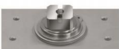
The NAMUR standard pinion groove and the NAMUR standard top mounting connection permit direct installation of accessories such as limit switch box and positioner
